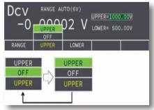
The comparator functions allows setting HIGH/LOW, and resistance and voltage can be simultaneously judged by independent comparators. Judgment results are provided on the display. External I/O is available for signal output.
